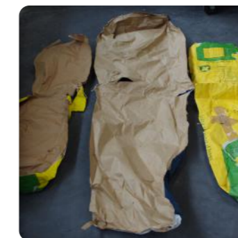
▶ Sacks are cut on 3 sides for a total opening and an integral emptying
