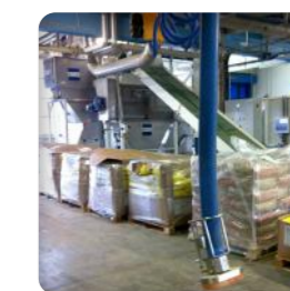
▶ Vacuum lifter to handle effortlessly sacks for an ergonomic working station (option)
