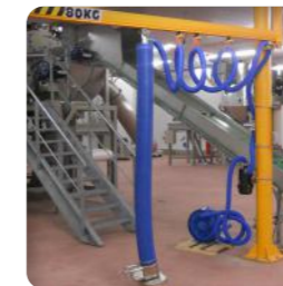
Vacuum sack lifter for an effortless loading of the machine. The rate is guaranteed with maximum ergonomics
