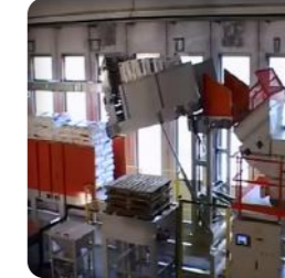
Automatic unstacker for a loading of the pallet without operator's intervention
