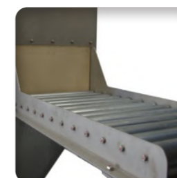
Roller conveyor to feed the machine
