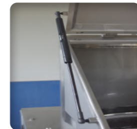
Gas cylinder to optimize the ergonomics and to support the door
