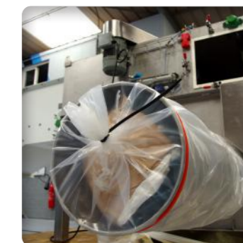
▶ Screw compactor to compact and discharge bags into a plastic sheath to secure the outlet of the compactor
