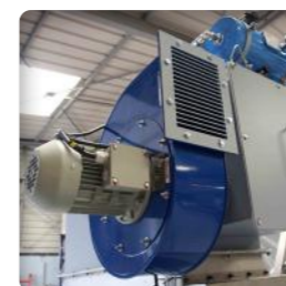
▶ Integrated dust collector
