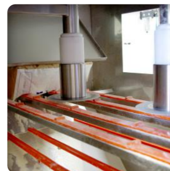
▶ Automatic cutting of the sacks for a rapid opening and increased productivity
