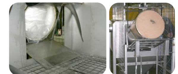
Lifting and positioning of the drum in the booth is performed by the elevator integrated on the booth
