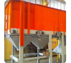
Vibrating chute to ease and control the flow of the material
