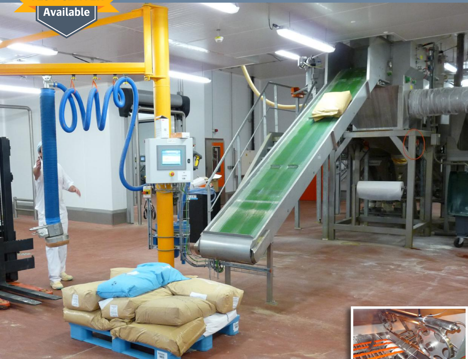
▶ The belt conveyor transports the bag directly to the ribbon-saw cutting system
