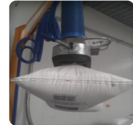
▶ Hessian bags: vacuum spike gripper to lift sacks of grains
