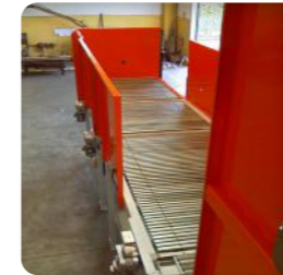
Sacks conveyor for the transport of pallets to the cutting system
