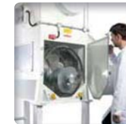
✂ Opening over the compacting screw
