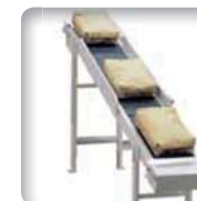
Inclined conveyor to feed the unloading station.
