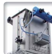
Dust collector ensuring healthy work environment
