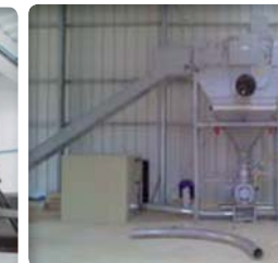
▶ Deconditioning of cement with pneumatic conveying
