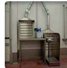
▶ Suction booth with integrated scale
