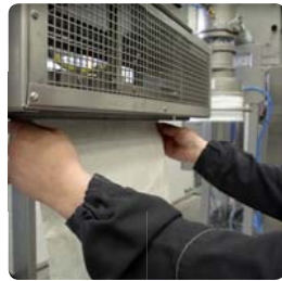
▶ Sack welder for a complete containment
