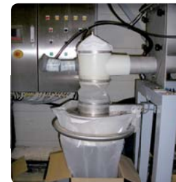
Sack filling for further conditioning to cardboards
