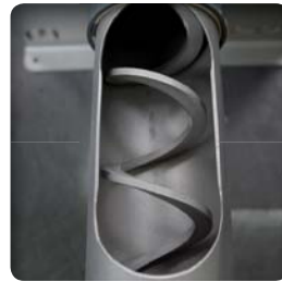
▶ Screw feeder for a high-accuracy dosing
