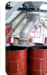
Connection lid with compression flange for filling on the pallet
