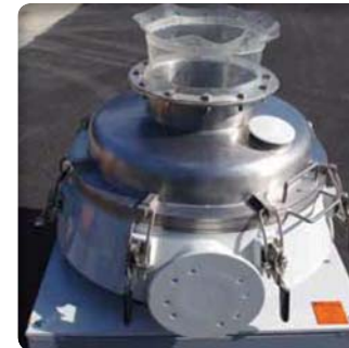
Entire vibratory sieve with flexible connection spout
