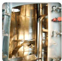
Polishing of welded components for hygienic finish
