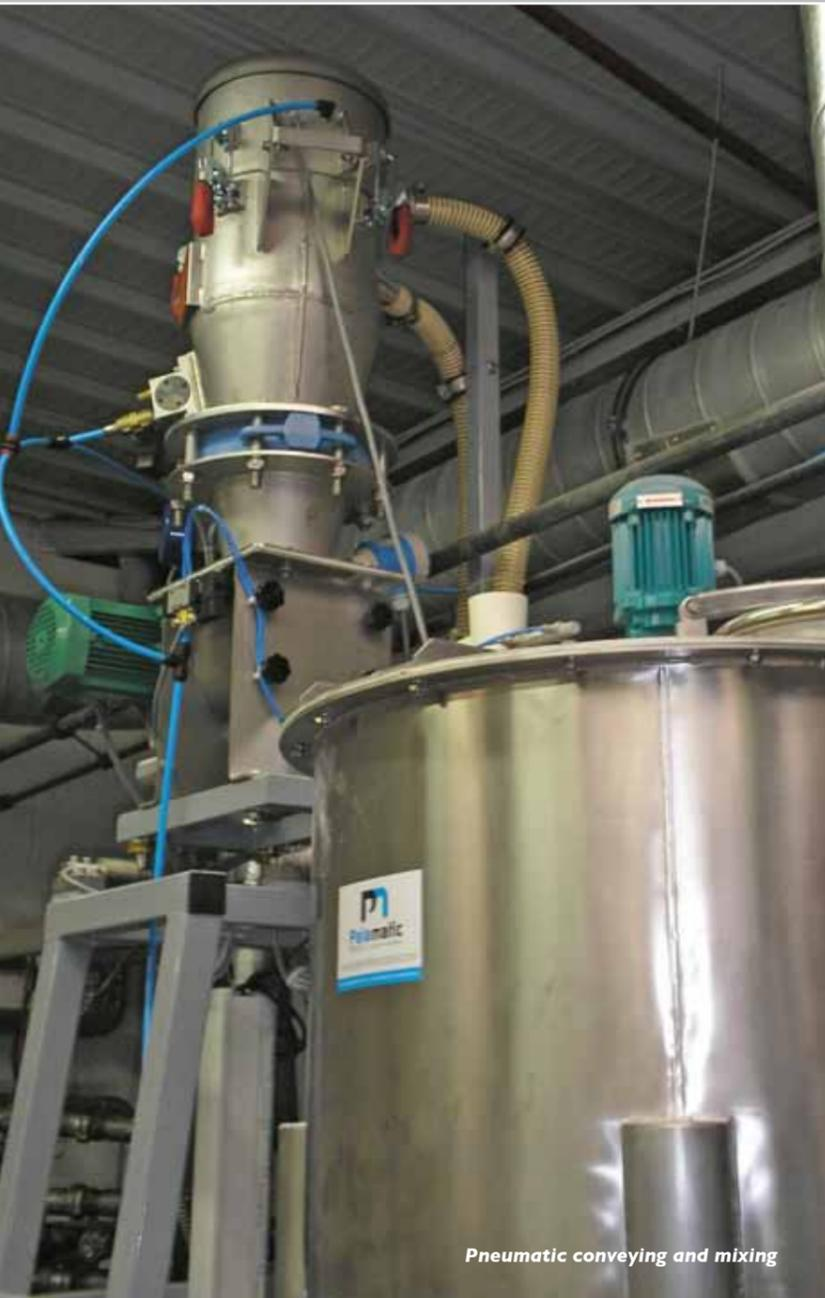
Pneumatic conveying and mixing
