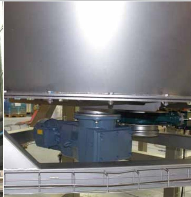
Vaults breaker on the bottom of the silo
